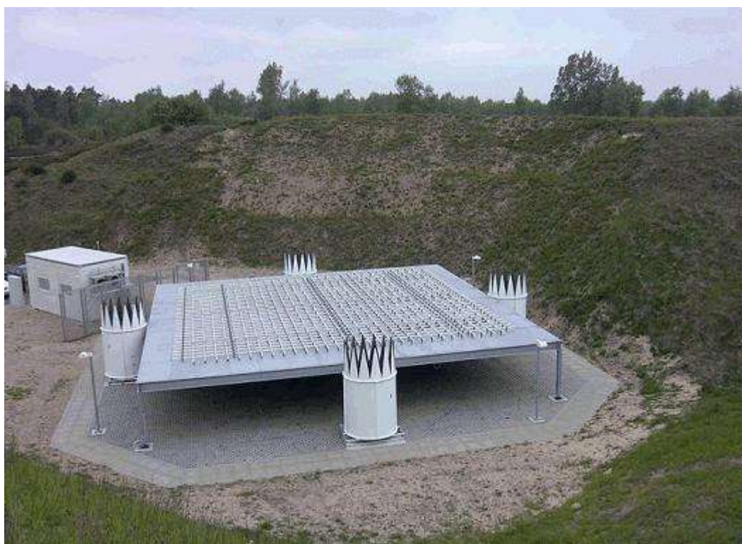
Fig.4.8 A schematic representation of a Wind Profiler
